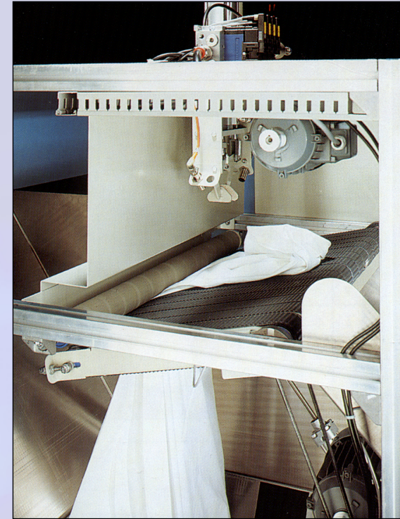
Conveyor belt moves against pressure roller and pulls out the item
