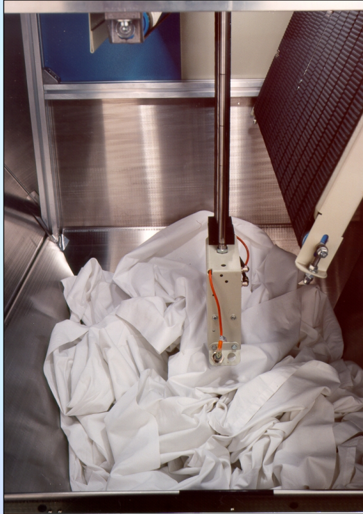
Sensor-controlled gripper takes out an item
