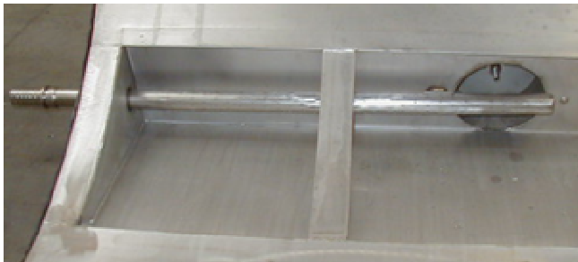
Direct Steam Injection
