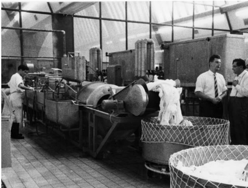
The first Poensgen Flowline Washer at test in a laundry at Krefeld / Germany –
