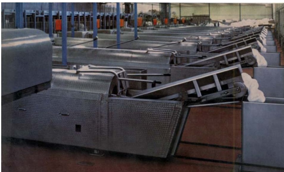
11 Tunnel Washers in the central laundry at Eskilstuna in Sweden standing side by side.
