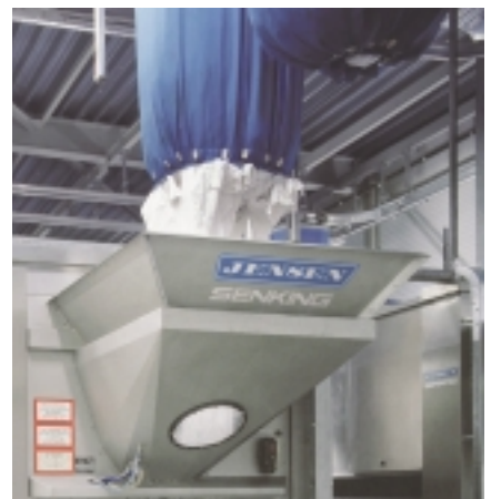
Precise batch size loaded directly into the wash tunnel.
