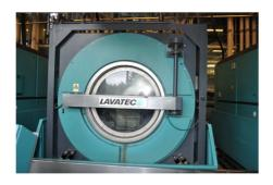
These two way tilting large washer extractors, known for their very heavy industrial construction, are currently used for washing of Dustmats but are certainly suitable for other applications like the processing of working gear.
