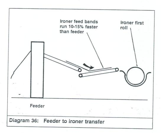
When an ironer is hand fed the highest feed rates are usually achieved if the work is pre-prepared and laid up on to a suitable trolley immediately behind the feeding point. The pre-prepared work is then generally flat with the correct edge leading, making for a much smoother feeding
