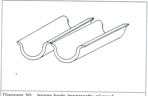
Diagram 30: Ironer beds incorrectly aligned
