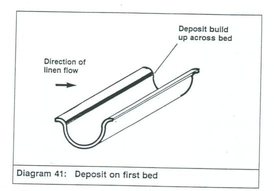
However, the main cause of deposits at the front roll is starch carry over. This can only be improved by attention to the starch rinse of the wash process and possibly by modification to the grade of starch used.
