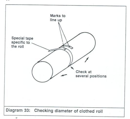
If the clothing is hard and compacted or if it is ridged or grooved, or if the surface is heavily charred, then the rolls should be reclothed - to delay this is false economy because it wastes production time and increases running costs.
