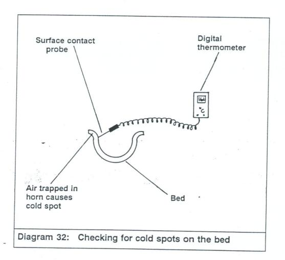
The measurement needs to be made at several points across each bed. If the systems are working correctly then all the temperatures should be within 2-3°C of each other with no cold spots and the average should be within about 5°C of the condensing steam temperature.
