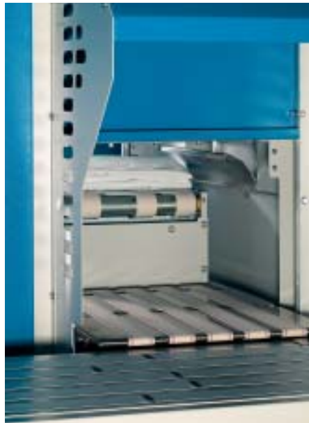
Lift stacker in transfer position
