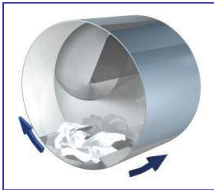
Oscillating washing action
